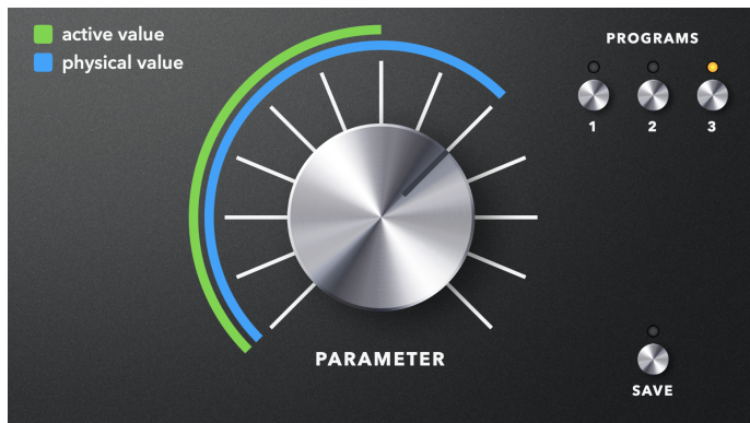
Fig. 1. The drawback with traditional, analog level meters. The physical and active values are out of sync!
